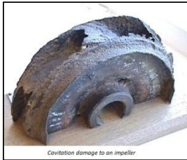
Figure 9: Example of cavitation
